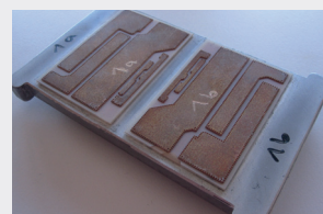
Elektronik Part AlN onto Al-Plate
